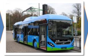
80% Fuel 60 % Energy reduction Electrical drive 70 % of route = silent 80-90 % CO2 reduction\* Charging 6 min at end stations.
