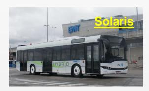
Consumption reduction: between 24 and 30 % (vs. Euro IV diesel bus)
